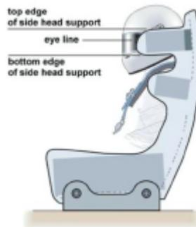
If a foam insert is used between the homologated seat and the driver, minimum lateral support to the driver's head, shoulders and pelvis must be guaranteed as follows:
