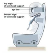
If a foam insert is used between the homologated seat and the driver, minimum lateral support to the driver's head, shoulders and pelvis must be guaranteed as follows:
